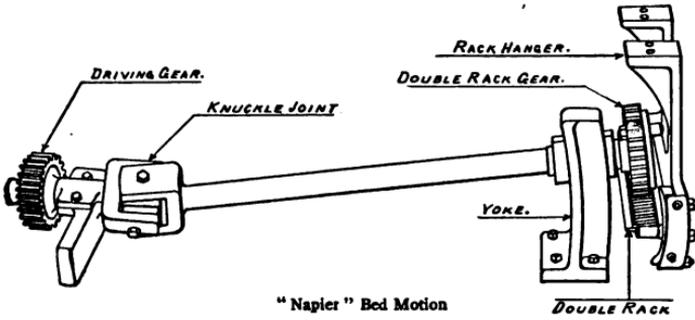
moves constantly in the same direction. When this gear is driving the rack from above the bed goes forward; at the end of the rack the gear drops below the rack and carries the bed back. It is possible to drive this gear in both positions because of a universal joint, or knuckle-joint arrangement, connecting the driving shaft of the press with the shaft driving the gear, called the intermediate driving shaft.
