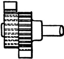
2. The driving gear may be double width, with the teeth cut away from certain portions of each half of the double width.
