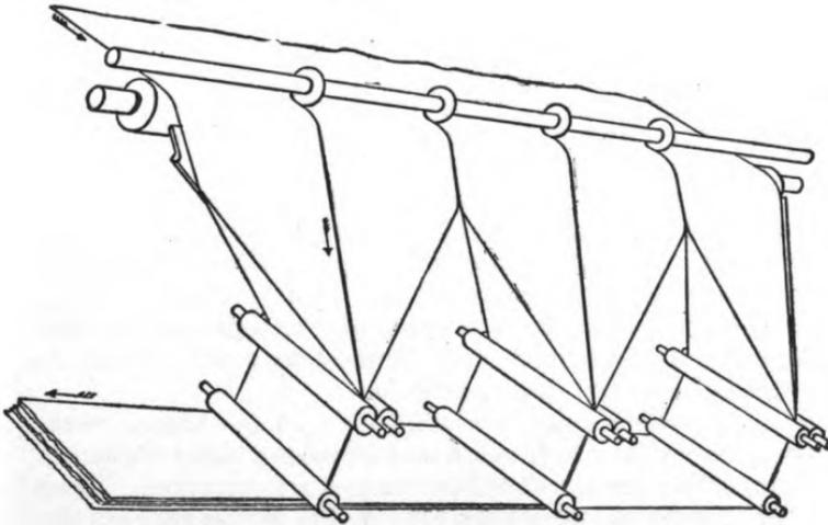
Illustration showing two formers and one half-former. Each former handles 8 pp., folded once; the half-former handles a single ribbon of 4 pp. The whole product of the machine is 20 pp. By leaving off one row of plates its product will be 16 pp. By separating the product of the two formers the mechanism will deliver two 8 pp. papers. By using the product of the half-former and one former, the press will deliver one 12 pp. paper.
