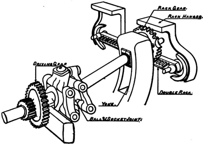
A Ball-and-Socket Universal Joint Bed Motion
