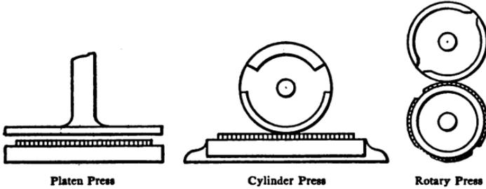
1. The platen press, having the type or form on a flat bed, the impression being given by a flat platen.
