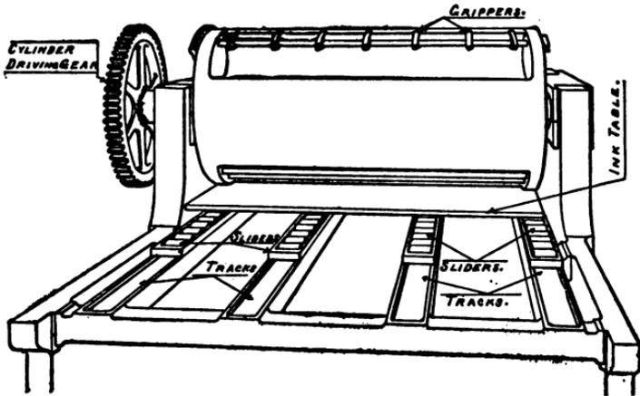
Two-revolution presses are usually provided with four tracks supporting the bed, sometimes with six tracks on wide presses.
