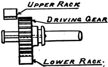
1. The racks may be set in different planes vertically, the gear sliding on its shaft.
