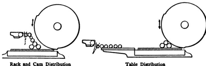
operated thereby. These rollers are set at an angle across the press so that they vibrate back and forth. This form of distribution makes a longer and less convenient press but is preferred for the better classes of printing as the distribution is better.
