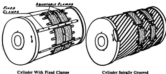
The simplest form of rotary press is the sheet-feed rotary, which prints previously cut sheets of paper one side at a time. It does the work of a flat-bed press but much more rapidly because there is no heavy bed and form to reciprocate. It may be a two-revolution machine with the
