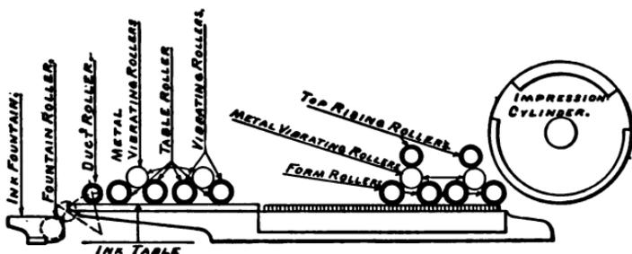
The above illustration shows the arrangement of rollers on a two-revolution press.
