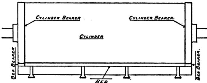
Two-revolution presses are provided with a wide bearer at each side of the bed, of iron or steel. They run in contact with similar bearers around each end of the cylinder. Their purpose is to ensure a uniform speed of movement between cylinder and bed, to lock them together as they were, to carry the cylinder over the spaces between pages,
