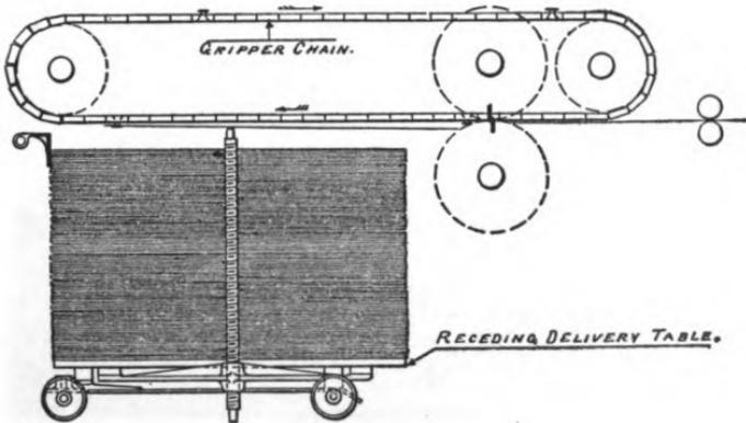
In case end grippers are used they are mounted on a bar attached to each end to this endless chain. As they come around in place they grasp the front end of each sheet and carry it forward to its proper place. The rest of the sheet is supported by rolls running in the white margins so as not to smut the printing.
