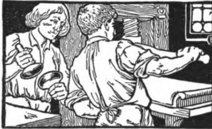
FIG. 1. Old-time Inking Balls, and Method of Use.
